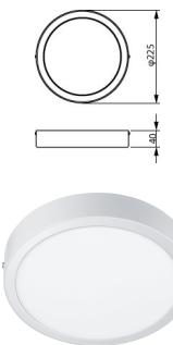
Scheda tecnica Philips Downlight LED Ledinaire G3 DN065C 19.5W 2000lm 110D - 830 Luce Calda - | 175mm
